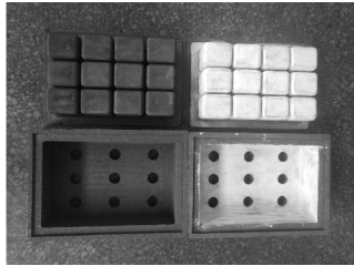
图 5 薄壁铸件的石墨型 Fig.5 Graphite mold for thin-walled casting
